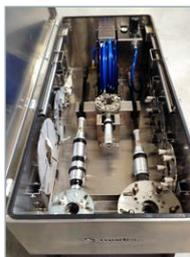
For **regular professional use**, the **modéc kit box** is a metal case that can hold all the equipment necessary for various operations (actuators, adaptors, torque management systems, batteries, chargers, FRL unit, air feed pipes etc). With the kit box, you can transport all the equipment to the work site **without difficulty** and **get started quickly and simply**.
